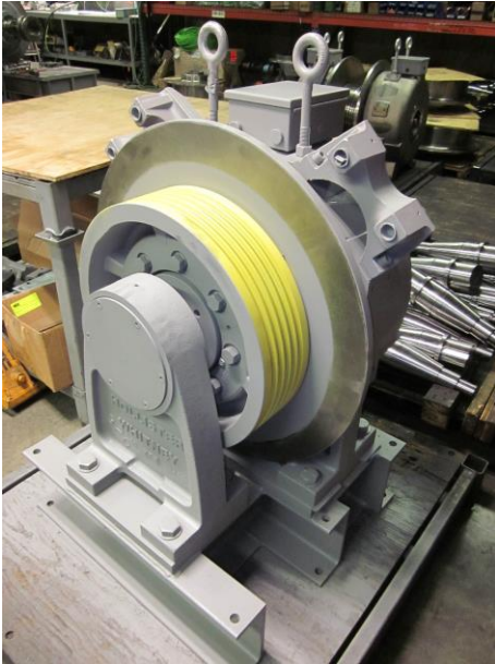
Figure 6 – GL171 with 2 lifting eye bolts installed
